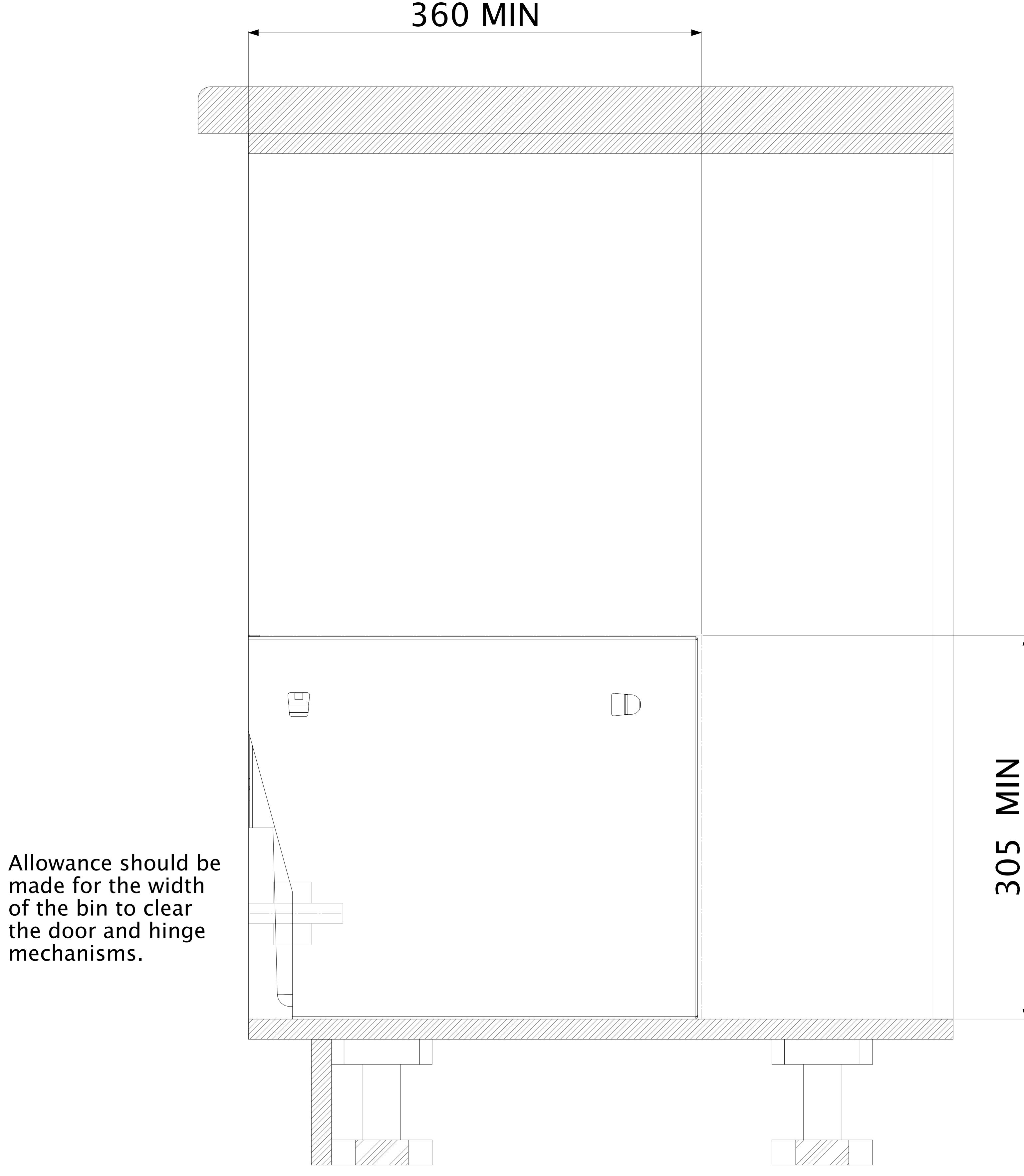
made for the width of the bin to clear the door and hinge mechanisms.
