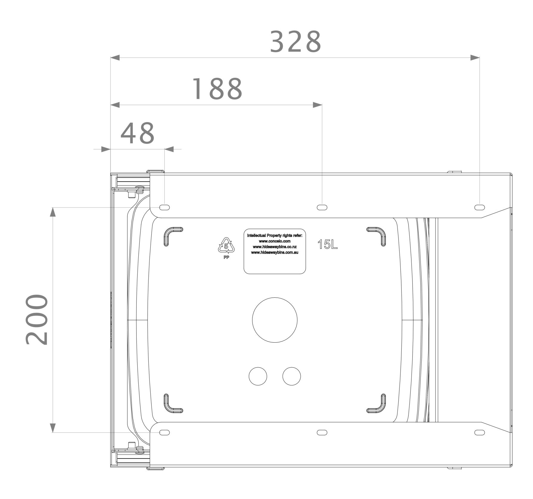
$\bigcirc$  2 x 10mm deep pilot holes required for mounting the body to the carcase with 16mm screws.
