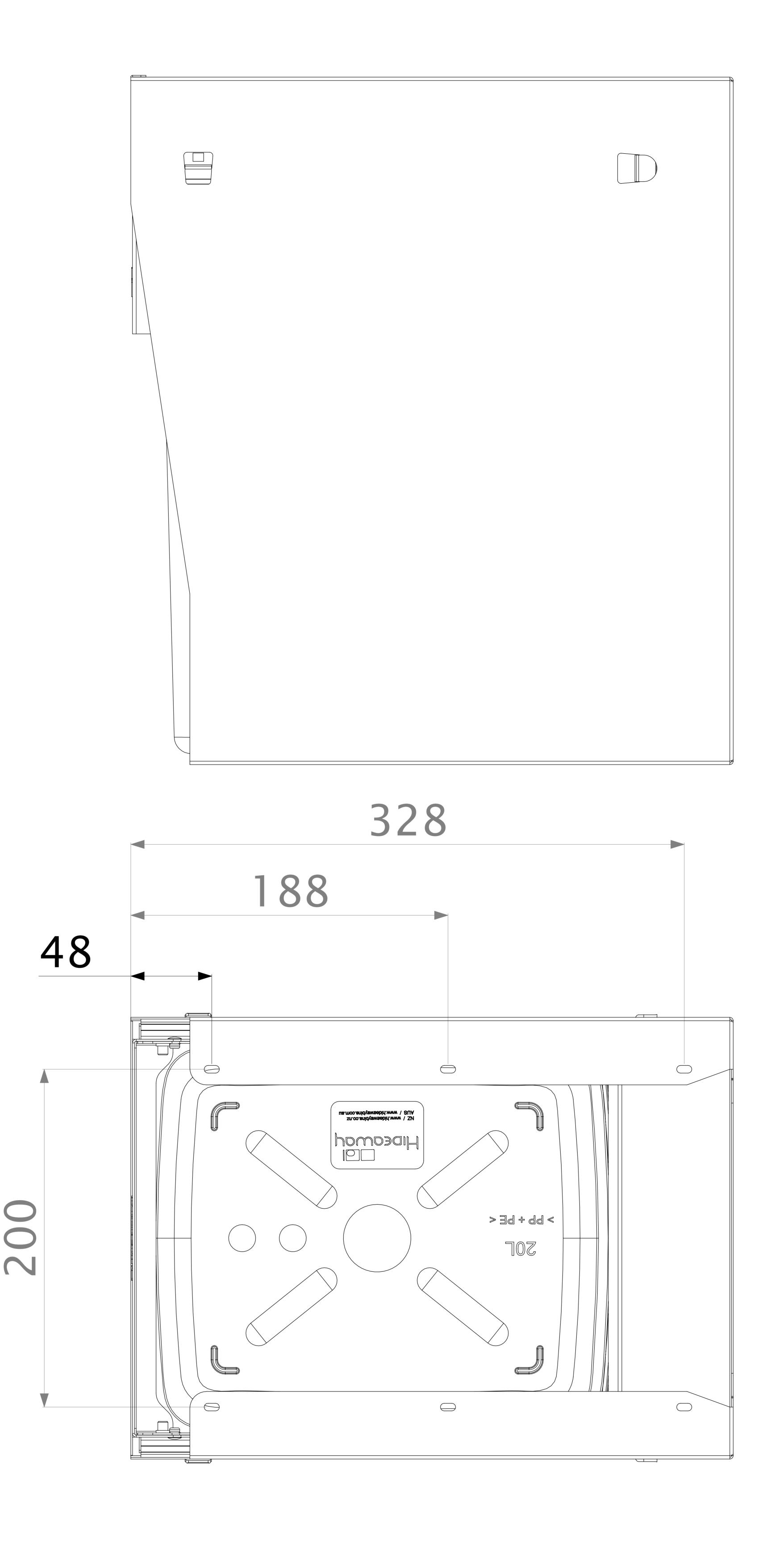
$\bigcirc$  2 x 10mm deep pilot holes required for mounting the body to the carcase using 16mm screws..
