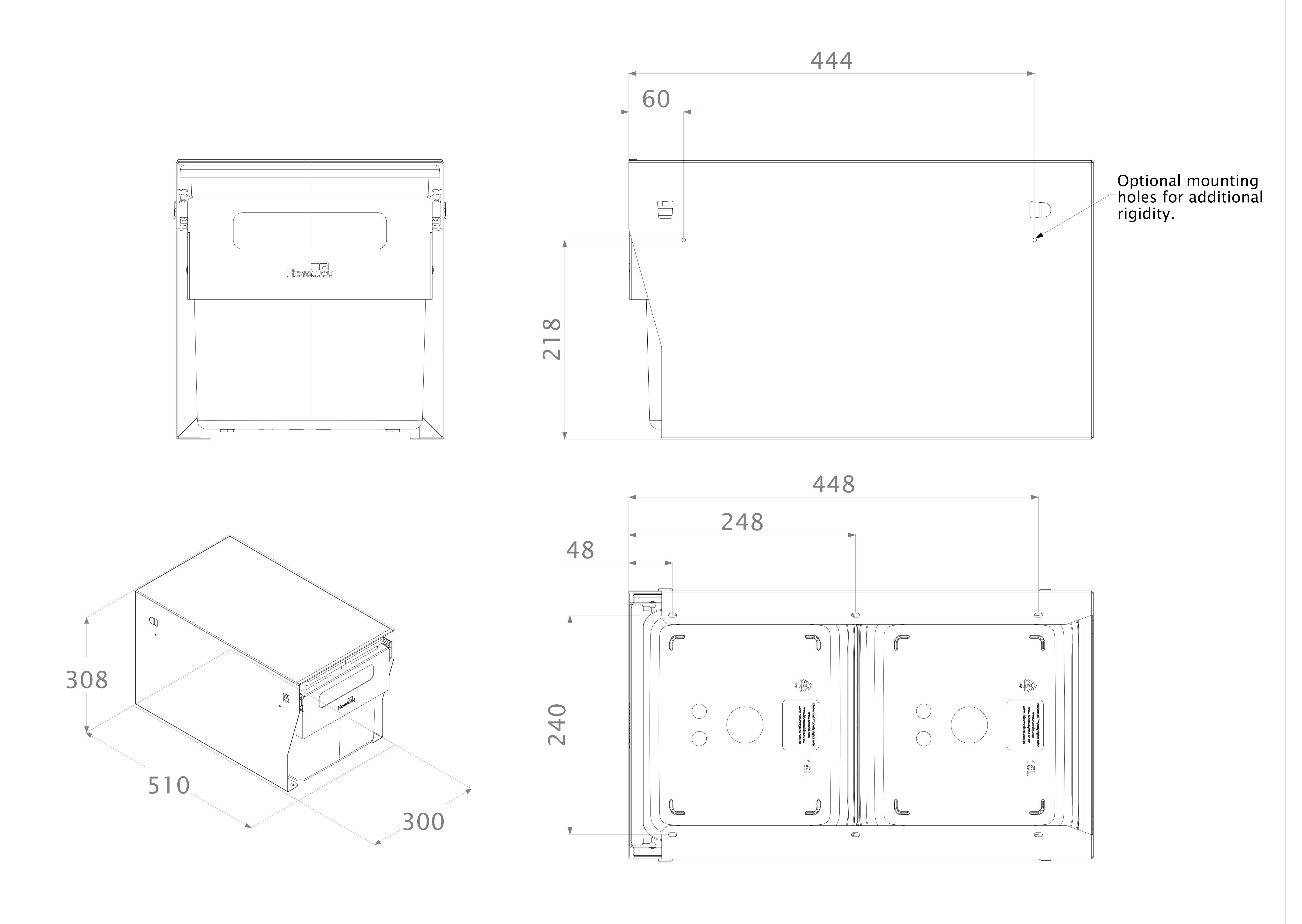
$\bigcirc$  2 x 10mm deep pilot holes required for mounting the body to the carcase using 16mm screws.
