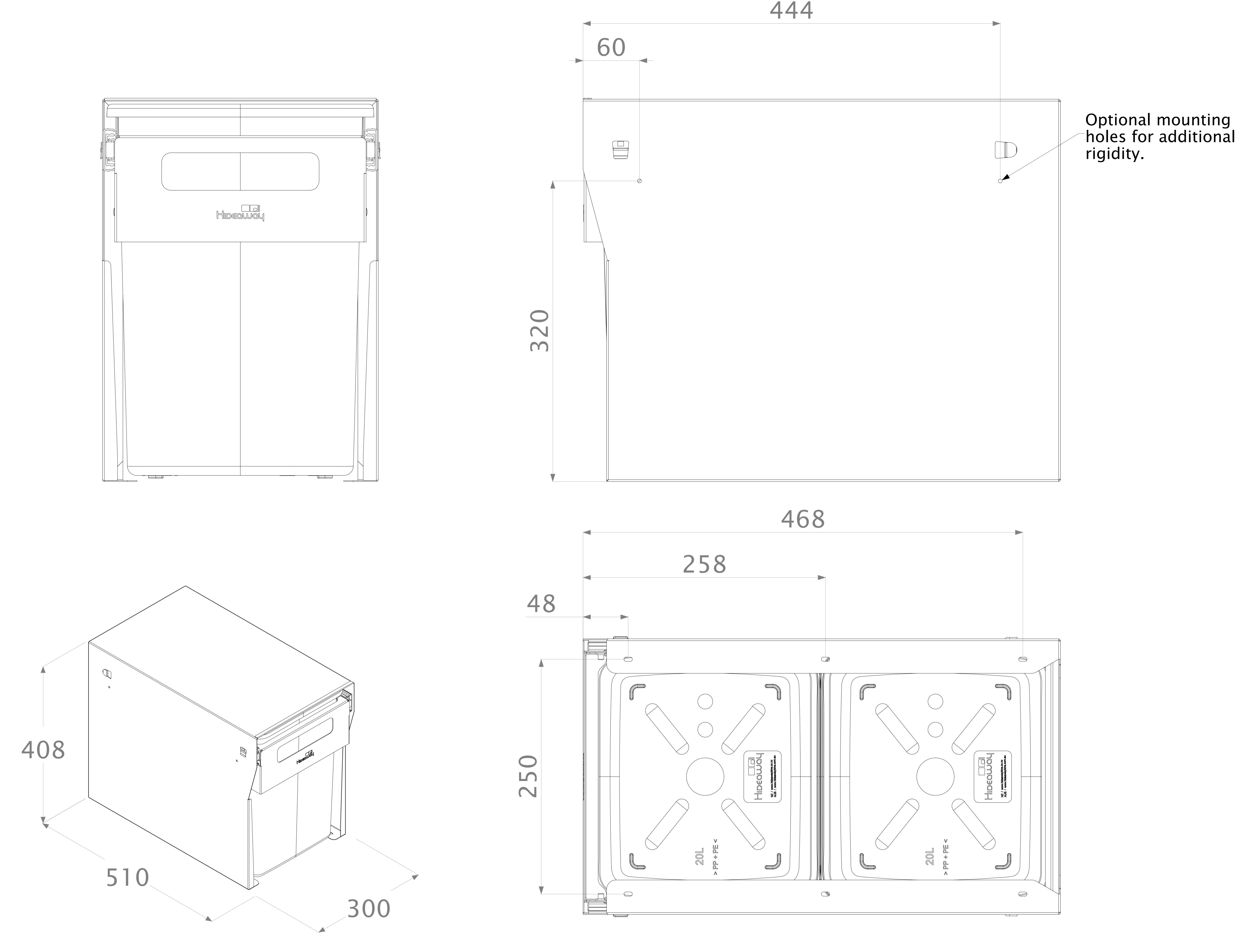
$\bigcirc$  2 x 10mm deep pilot holes required for mounting the body to the carcase usinmg 16mm screws.
